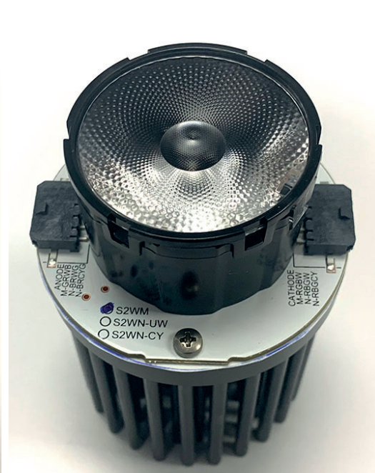
Light engine without wire harnesses
